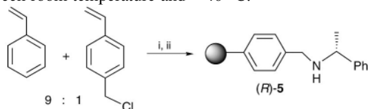
Scheme 3 Reagents and conditions: i, AIBN, toluene, 70 °C, 40 h; ii, ( R )- \alpha -methylbenzylamine (3 eq.), NaI (1 eq.), DMF, 48 h.
